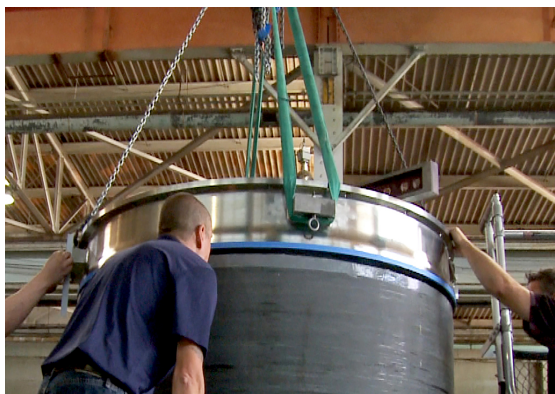
OceanGate Director of Engineering Tony Nissen verifies that the titanium ring is perfectly aligned to the carbon fiber hull.
