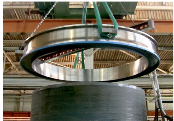
Titanium ring is lowered precisely to the carbon fiber hull prior to permanently bonding the two major components of Cyclops 2.
