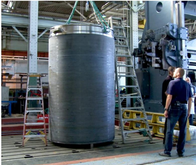
Workers survey the scene after a titanium ring is placed on the carbon fiber wound cylinder for Cyclops 2's pressure vessel. (OceanGate Photo)
